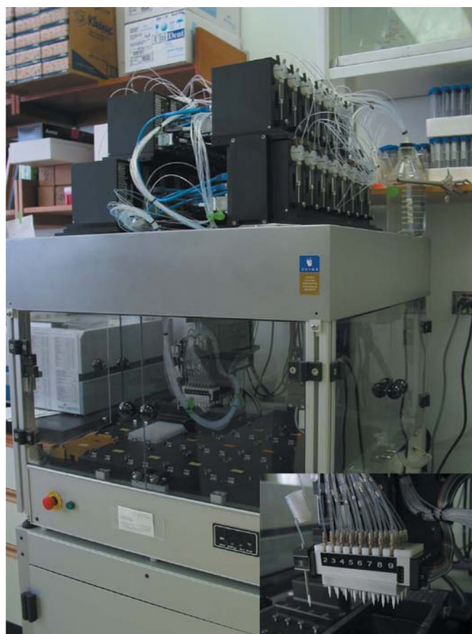
Figure 2 Image of the Honeybee robot (Genomic Solutions) with the syringes on top of the humidity-controlled cabinet that holds the plate deck, sample and wash stations and the dispense heads. An enlargement of the 32 reagent dispense heads and one extra protein dispense head is shown in the bottom right corner.
